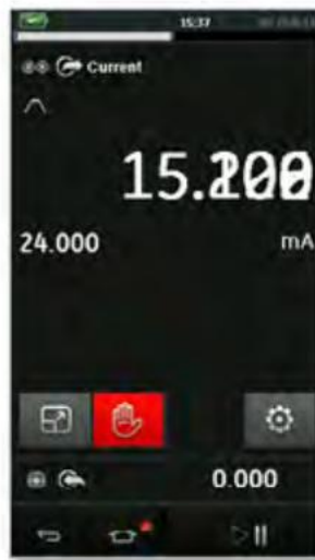
RAMP automatic cycle
