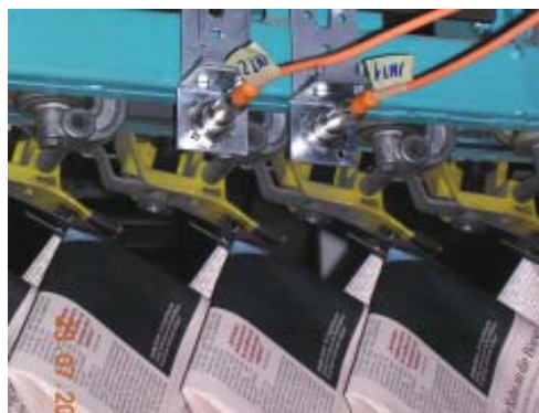
Picture 8 Counting of number of folds of paper filter elements (LCC-CON1)
