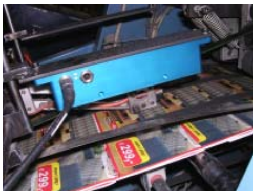
Picture 5 and 6 Copy counting during overhead conveyance (LCC-90, LCC-90-MA)
