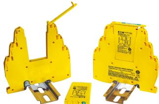
**The MTL SD modular** range takes the established SD range of high performance surge protectors for I/O and introduces a replaceable element. Maintaining the unrivalled packing density and field proven hybrid circuit design the modular range makes maintenance easy, enabling the replacement of surge protection modules without disconnecting the loop.
