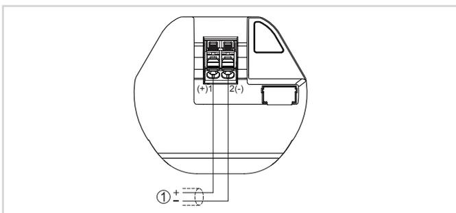
Compartiment de raccordement VEGAPULS 21
