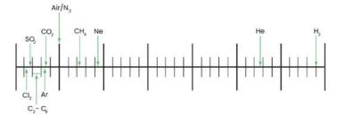
Note: Graph is relative thermal conductivity at 212°F (100°C)
