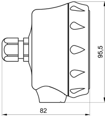
FlexHousing with bottom process connection
