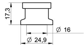
Tri-Clamp Ø 24.9, membrane Ø 16 mm (BCID: C01)
