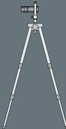
Blackbody Accessory 798-05-02 This accessory allows the calibration of infrared (IR) thermometers
