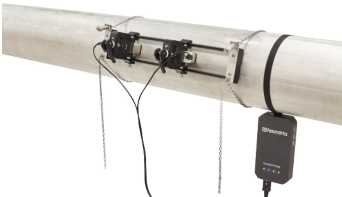
Clamping fixture, transducers and transmitter mounted on pipe
